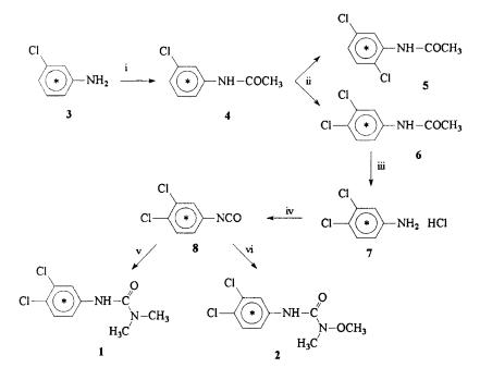
i = acetic anhydride, acetic acid, room temp., overnight; ii = N-chlorosuccinimide, acetic acid, 2 days at room temp., then 2 h at 60°C; iii = conc. HCl, ethanol, 2 h reflux; iv = trichloromethyl chloroformate, benzene 2 h reflux; v = dimethylamine, dichloromethane, 2 h at room temp. vi = N, O-dimethyl hydroxylamine, dichloromethane, 2 h at room temp.
