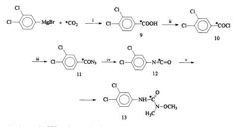
i = ether, r.t.; ii = SOCl<sub>2</sub>,, reflux, 2 h; iii = NaN<sub>3</sub>, acetone, 3 h, r.t.; iv = toluene, 80-100°C, 2 h; v = N,Odimethyl hydroxylamine, dichloromethane, 2h, r. t.
